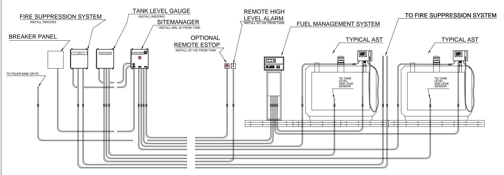
\* INSTALL THE SITEMANAGER DUTDOORS 20 to 100 FEET AWAY VISIBLE FROM THE FUELING AREA. IF INSTALLED INDOORS OR NOT VISIBLE FROM THE FUELING AREA, AN ADDITIONAL REMOTE EMERGENCY STOP BUTTON MUST BE USED
